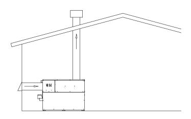
Figure 14 – Sidewall Combustion Air Inlet
